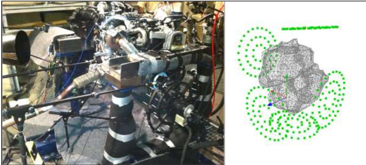
Figure 6. Engine in the test cell (left), mesh with the measured array positions (right)
