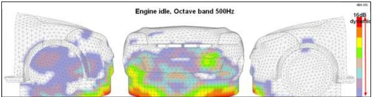
Figure 11. Intensity hologram for octave 500Hz, engine is idle, right face (left), front face (middle), left face (right)
