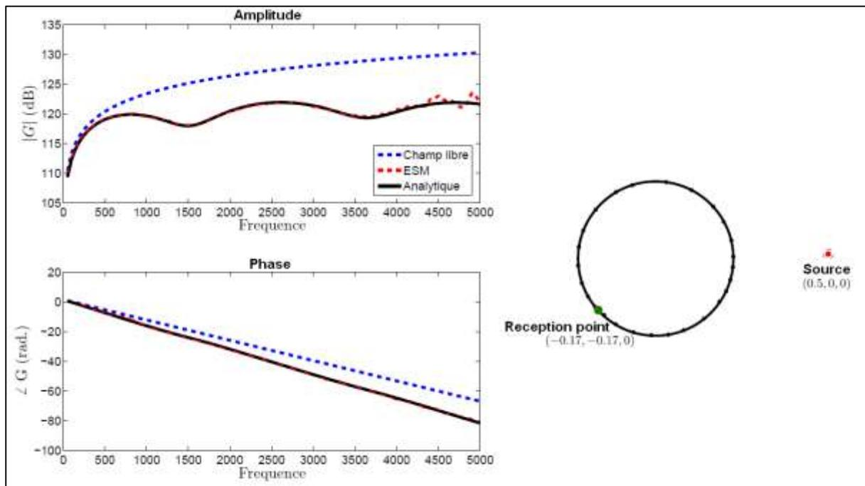
Figure 3: Numerical validation of ESM applied to rigid sphere case. Blue is free field result, red is ESM result, black is SRTF result (reference)
