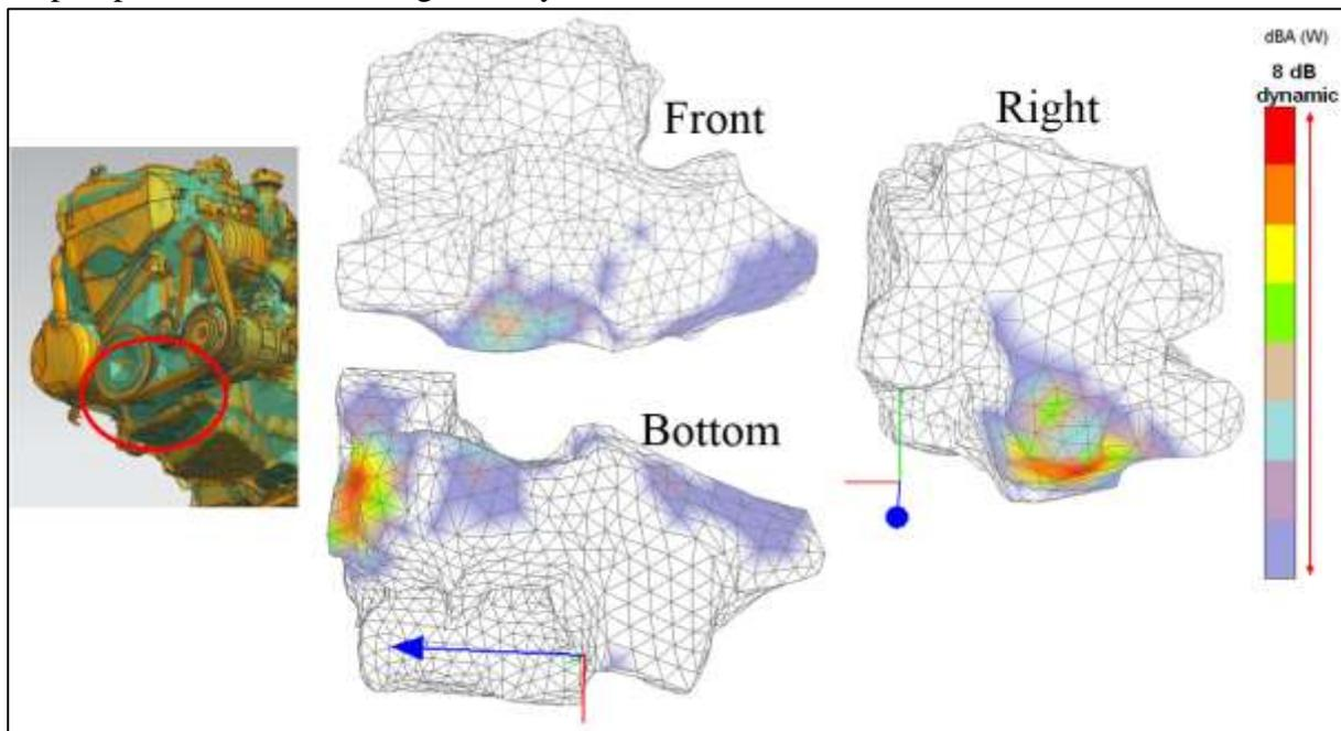
Figure 7. Intensity hologram at 2 kHz for different faces view, full torque, third gear.
