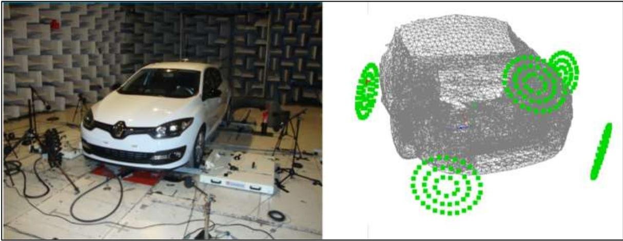
Figure 9. Car on the dyno (left), mesh with the measured array positions (right)
