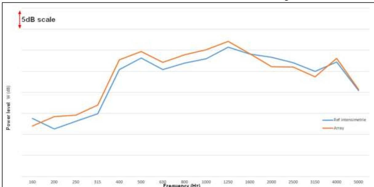
Figure 8. Power level comparison, partial torque-4<sup>th</sup> gear, between intensity probe (blue), and Generalized Acoustic holography (orange)
