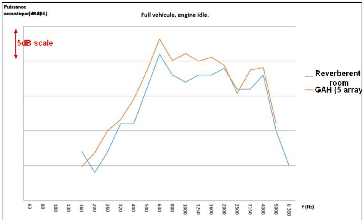
Figure 10. Power spectrum comparison, full car, idle state, measured in reverberant room (blue), and with generalized acoustic holography (orange)
