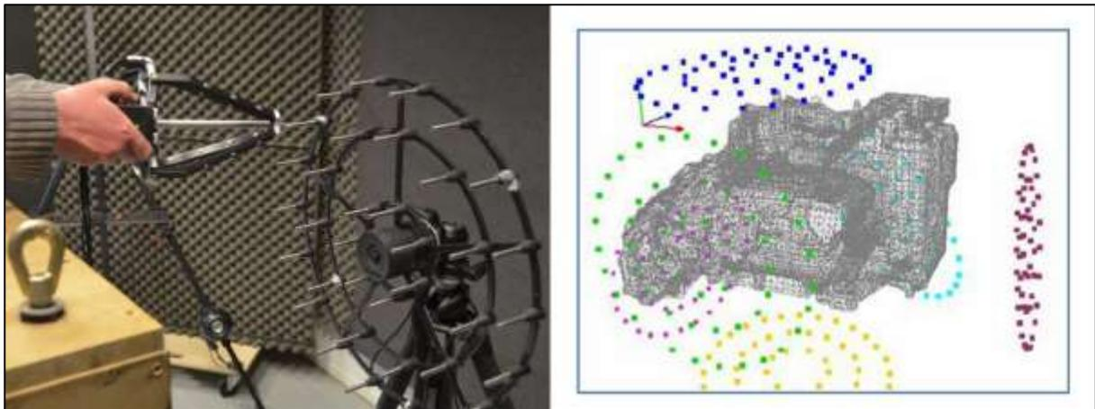
Figure 2. Positioning device (left), and mesh example with array setup (right)
