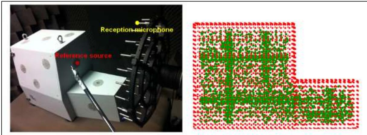
Figure 4. Engine mockup, and test setup ((left); Numerical model with equivalent source in green color (right)
