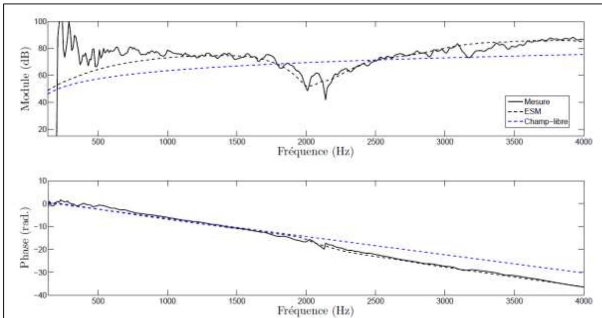
Figure 5. Module and phase of the transfer function (setup fig 4), measured (solid black), simulated with ESM (dotted black), and free field (dotted blue).
